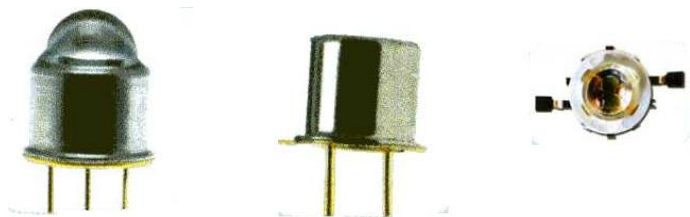
Figure E2: Examples of LEDs with dome lens and flat lens ( www.biouvled.com )
